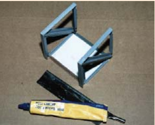
2. The platform and girder supports are glued together on a flat surface to ensure they set completely square.
